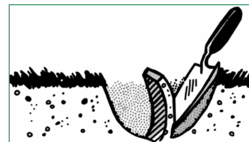
Figure 3. Soil sampling with a trowel.
