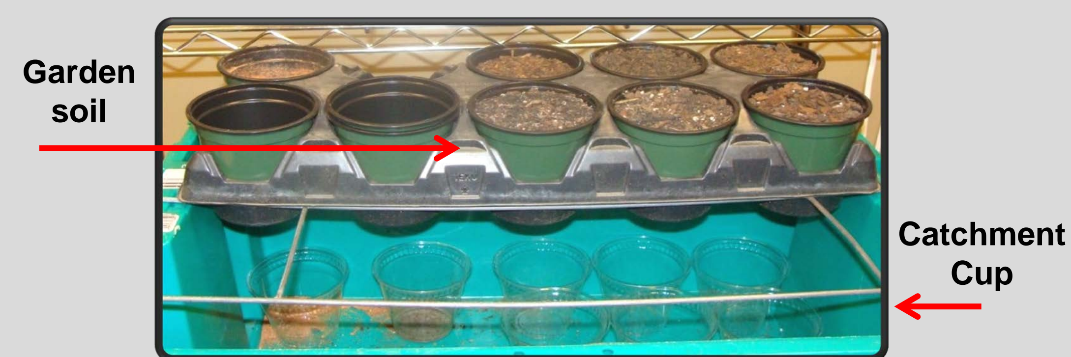
Figure 1. Set-up to measure soil's relative moisture characteristics
