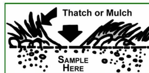
**Figure 2.** Remove grass thatch or mulch before sampling.
