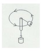
**4.** What is the force pulling the 100 gram mass down? This is the same force that is pulling the stopper inward. Show your equation, answer, and units below (Remember the unit for Newton is kg·m/s²).
