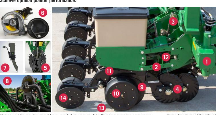
Always consult the operator's manual for the manufacturer-recommended settings for planter components such as vacuum, downforce, and closing wheel pressure to obtain optimal field performance. Properly lubricating all moving parts will help ensure efficient planter operation and extend the life of planter components.
