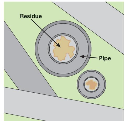
**Corrosion** is caused when water reacts with or dissolves metal plumbing. This can add toxic levels of metals like copper and lead to your water. Other problems associated with corrosive water include:
